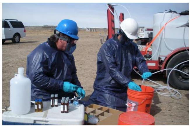
EPA workers in protective gear obtain samples for studying groundwater contamination in Pavillion, Wyoming. US EPA
