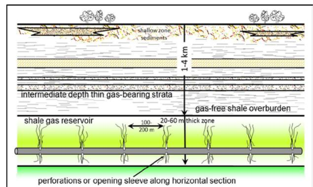
Figure 3. Schematic of vertical fracture propagation as a function of depth of stimulation. Note the presence at an intermediate depth of thin gas-bearing strata.
