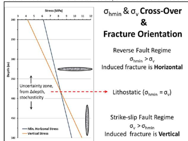
Figure 6. The orientation of fractures, stresses and gradients, Milk River Fm., north of Medicine Hat, Alberta
