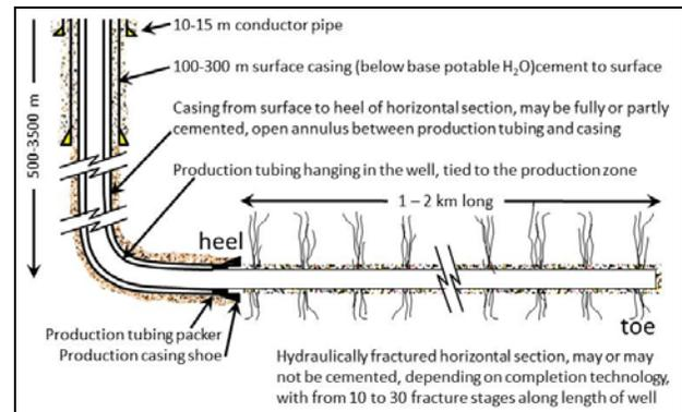
Figure 2. Schematic of the heel and toe of a horizontal well that has been hydraulically fractured
