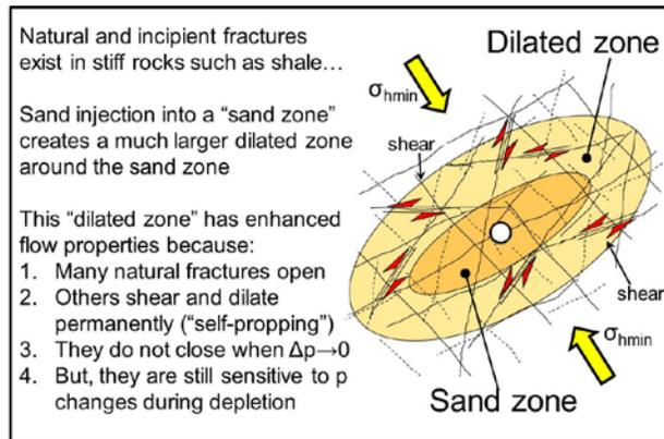
Figure 5. The stimulated rock volume (SRV or SV) is the total volume of rock mass surrounding the fracture point where enhanced transmissivity has been generated.
