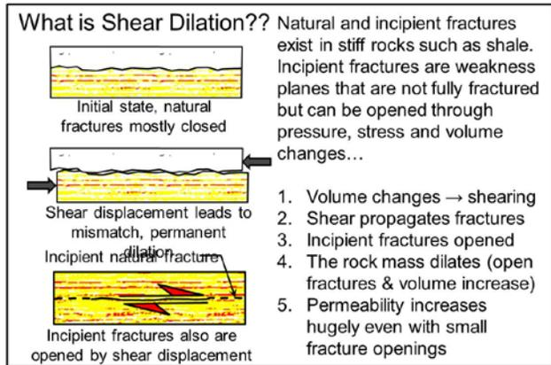
Figure 4. Shear dilation enhances the flow capacity of the shale gas rock mass
