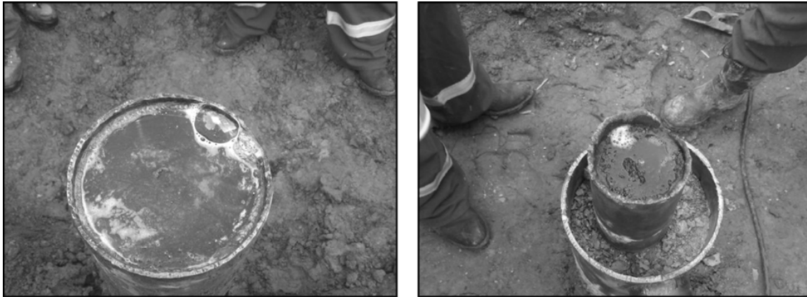
Figure 7: Illustration of leaking casing caps found at wellbore re-entry on surface casing and production casing.
