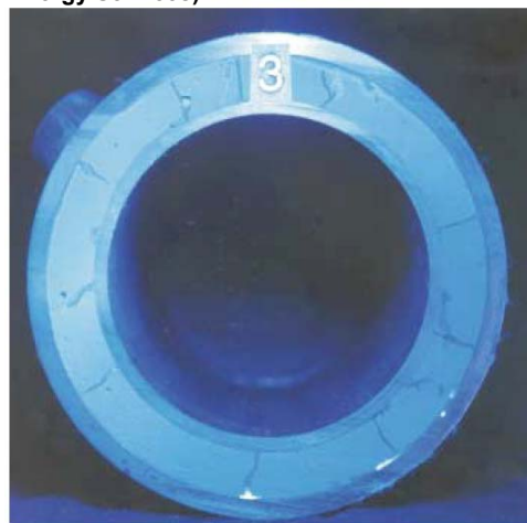
Figure 4: Cement sheath failure and resulting cracks developed from pressure cycling the internal casing (Watson et al., 2002). (Photo courtesy of Halliburton Energy Services).
