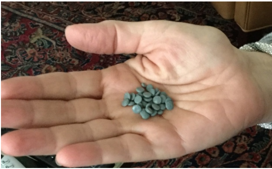
Plastic pellets (aka “nurdles”) are produced in the cracker plant. These will be shipped to other facilities to be formed into plastic products – from drain-pipes to water bottles. Photo by Vera Bonnet
