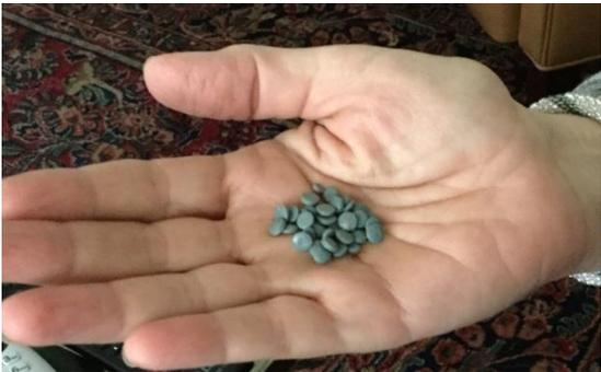
*Plastic pellets (aka “nurdles”) are produced in the cracker plant. These will be shipped to other facilities to be formed into plastic products – from drain-pipes to water bottles.
